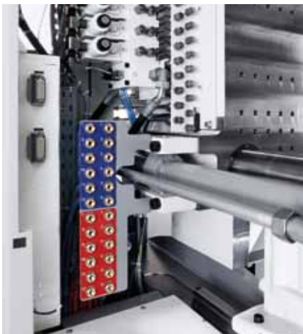
All of the important interfaces for the mold can be reached easily
